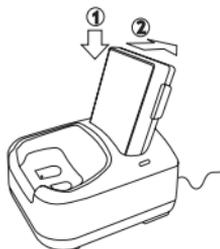
**'Dual Desktop' charger:** position the battery as shown in the drawing: 1- place the battery in the cradle, 2- press down backwards until it clicks into place
