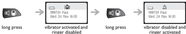
This key can be used to switch rapidly from the ringer to the vibrator and vice-versa.
